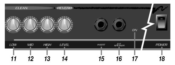
**16: EXT. SPEAKER:** Use this jack to connect an extension speaker cabinet to the amplifier. This jack is wired in series with the internal speaker(s).
